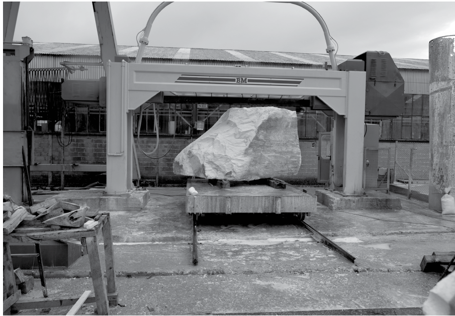
FIG. 3.4 Monowire diamond saw at Mount Pentellicus. Photograph by the author, 2025.
