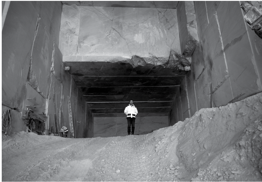
FIG. 3.5 Subterranean extraction of Pentelic Marble. Photograph by the author, 2025.
