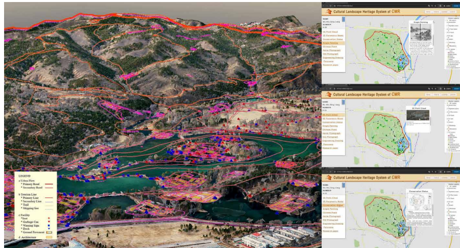
FIG. 3.4 A (left): 3D modeling of point clouds in GIS used as the basis of our study; B (right): Web-GIS platform for unified retrieval and management of the CMR.
