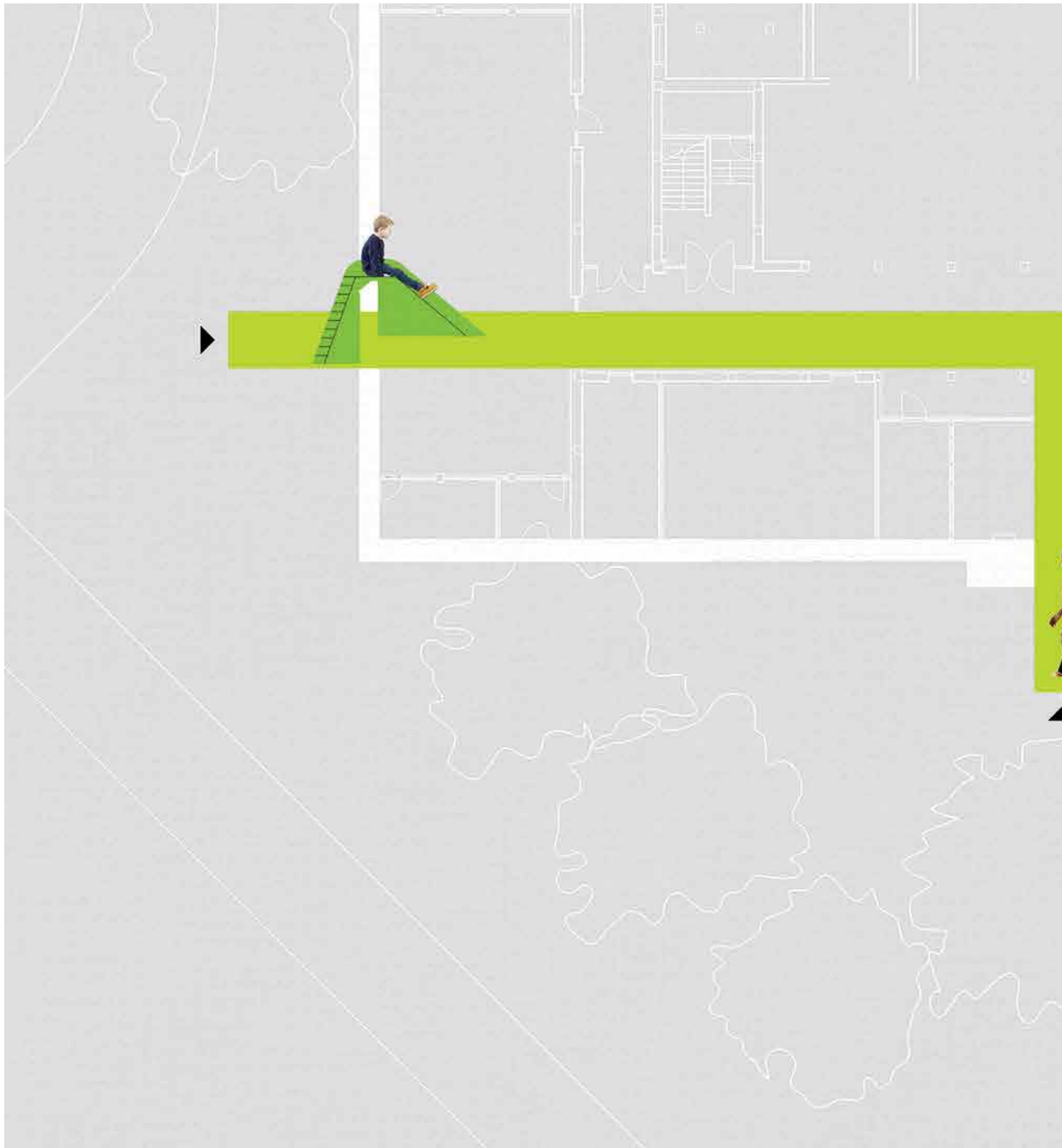
FIG. 5.12 The spatial intervention proposed an inner street crossing the building's entrance hall accessed through two slides in opposing windows and connected by a colourful carpet extending into public space.
