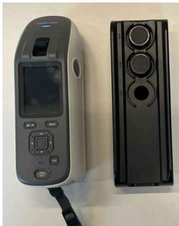
FIG. 5.2 Ground-truth measurement setup: reflectance spectrophotometer and its calibration module.
