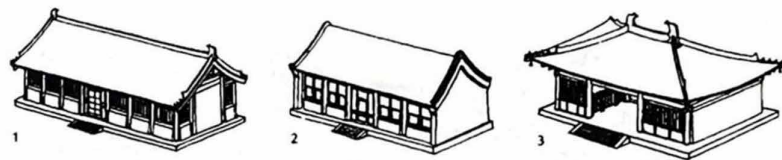
FIG. 4.18 The roof ridge changes from short to long (Sicheng Liang)
