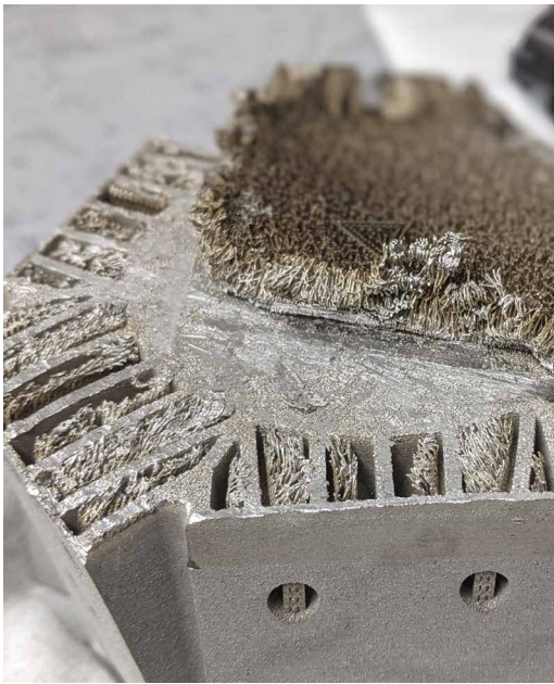
FIG. 4.24 PBF-L node with difficult to remove support structure (Image by author)
