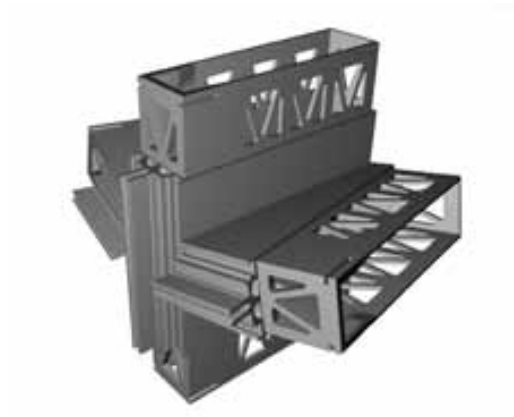
FIG. 3.3 Rendering of Nematox I façade node by Holger Strauss [129]; the first AM structural node for freeform metal and glass construction. Design for stick-built aluminium façade system and equipped with standard connections, and integrated screw channel and gasket rebates. (Image source: [129])
