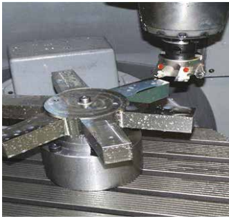
FIG. 2.6 CNC-machined node with simple geometry from DZ Bank Berlin (Image source: [113])
