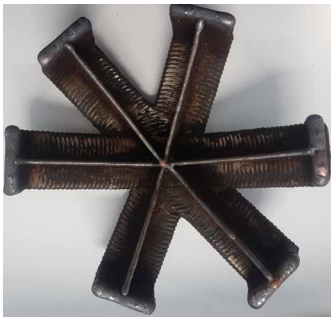
FIG. 6.17 Preliminary prototype for DED-GMA node with excessive warping (Image courtesy of Mx3D)
