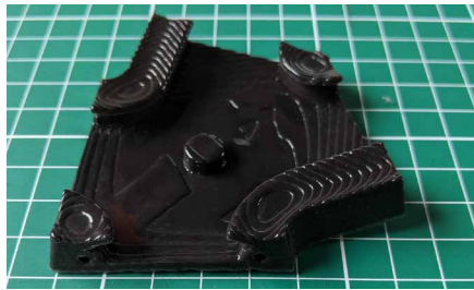
FIG. 5.6 Gasket prototype printed in Silicone GP Shore A 60 by ACEO using drop on demand printing technology. (Image by author)
