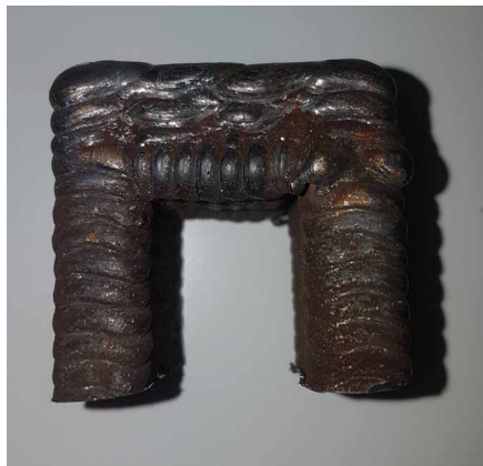
FIG. 6.22 Sample iteration of end condition using less material but more complex path planning that requires several changes of printing orientation which are visible in the surface texture (Image courtesy of Mx3D)
