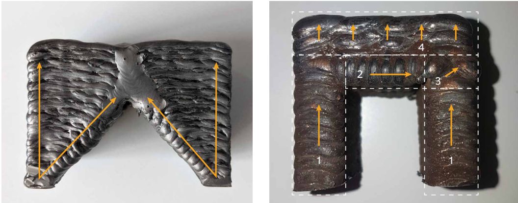
FIG. 4.30 End connection alternatives explored during the development of DED-GMA node: increasing thickness with simple path planning (left) and flat end face with multiple steps and orientations (right). (Image by author w/ photo courtesy of Mx3D)
