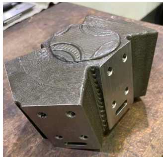
FIG. 6.18 Preliminary prototype for DED-L node with undesirable surface texture (Image by author)
