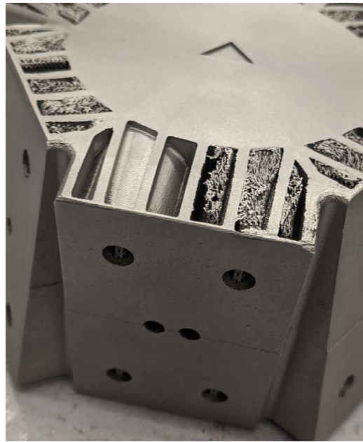
FIG. 4.25 Leftover support structures after removal effort with CNC milling (Image by author)
