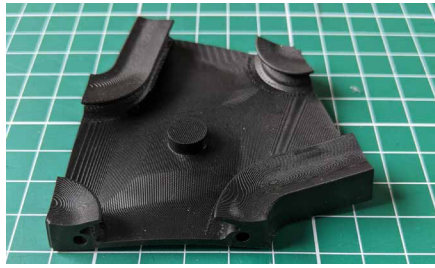
FIG. 5.4 Gasket prototype printed in EPU 40 by Sculpteo using digital light synthesis printing technology. (Image by author)
