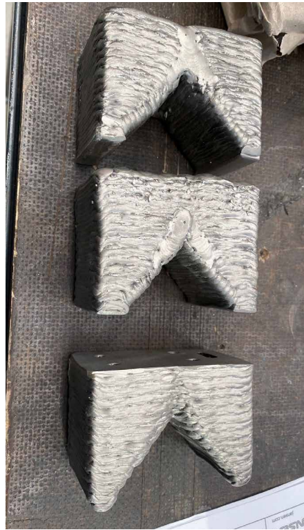
FIG. 6.21 End-condition iterations to improve surface quality by integrating contour paths, printing solid end conditions without integrated boring holes, and subdividing the path planning for the solid infill (Image courtesy of Jansen AG)
