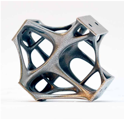
FIG. 3.7 3D Printed stainless steel node for steel and glass canopy, prototyped at 25% scale using BJ. (Image source: [4])
