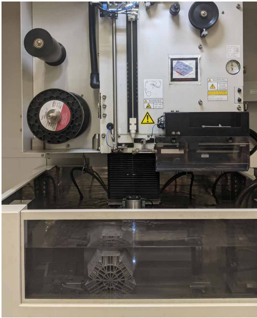
FIG. 4.22 EDM process on PBF-L node (Image by author)
