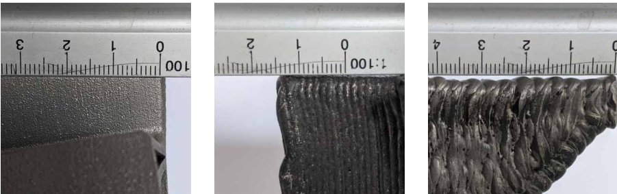
FIG. 4.26 Relative surface roughness of PBF-L node (left); DED-L node (middle); and DED-GMA node (right). (Image by author)
