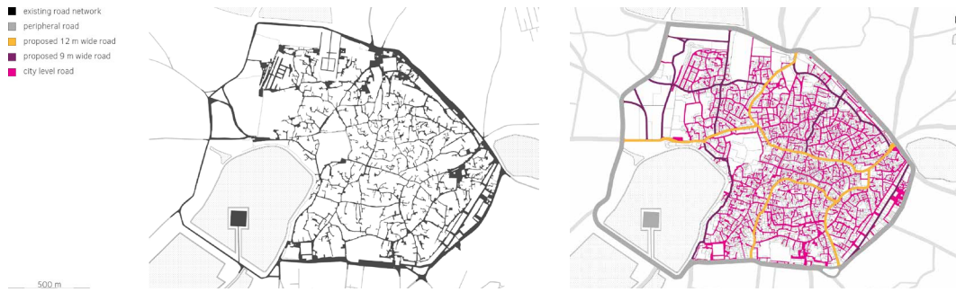
FIG. 4.8 Town Planning Scheme (TPS) with road network adjustments by land pooling for the walled city of Bhuj: (left) the road network of the walled city before the TPS; (right) the new road network with higher road density and reduced block sizes after the TPS (HCP, 2004).
