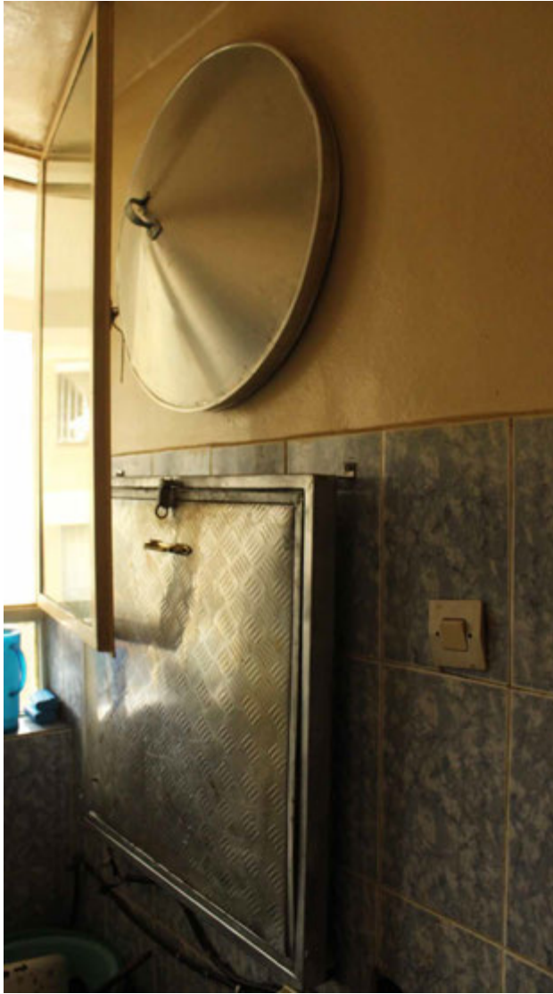
FIG. 5.25 Foldable injera stove to save valuable kitchen space in the condominium.
